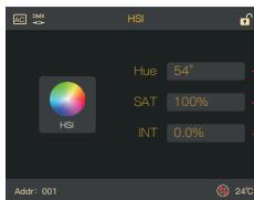
Hue, switch the CCT/Hue knob to adjust from 0° to 359°
