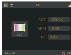
CCT, switch the CCT/Hue knob to adjust CCT from 2700K to 10000K
